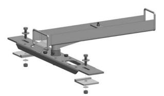
Swivel arm to be applied on the rear side of the Tractor Unit. It allows the hoses to follow the semitrailer's movements, without the necessity of using additional fittings. Painted with grey RAL 7021 epoxy dust, it has a complete steel structure and it comes complete with greaser for helping the maintenance operations.
